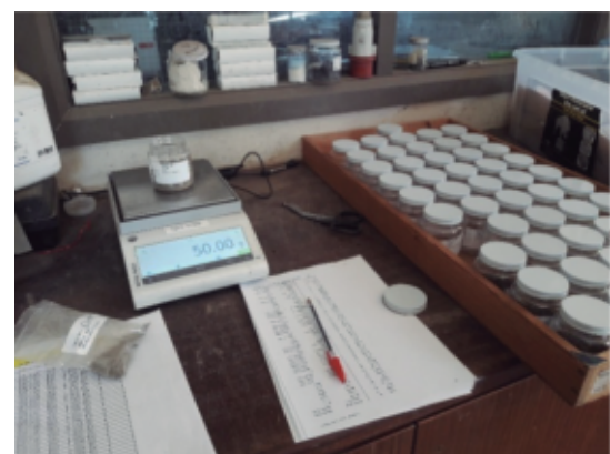
Picture 2: Preparation of soil samples collected from cross border catchments, for Morgan and Olsen soil P test comparison
