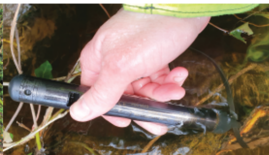
Figure 4 A data logger being installed in a spring
