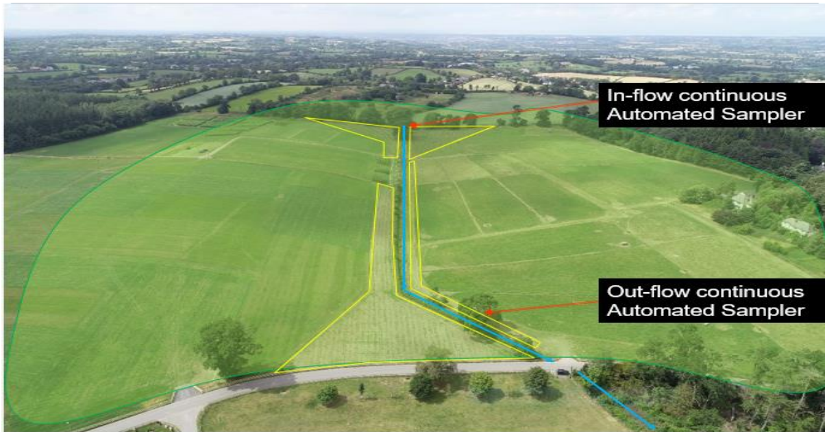
Figure 2: Highlighted areas indicating zones for willow planting with position of water samplers
