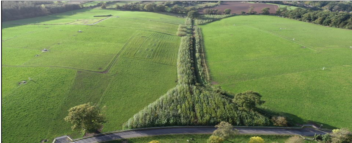
Fig 3. Biofiltration block protecting waterway from diffuse pollution.
