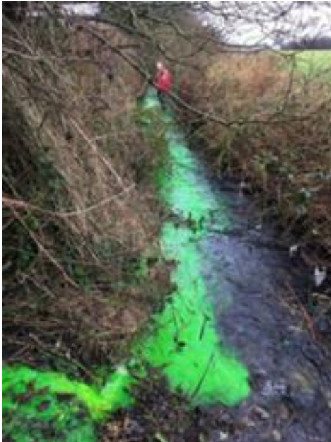
Figure 7 - Dye-tracing at Liscooley showing the WWTW discharge point on the left bank.
