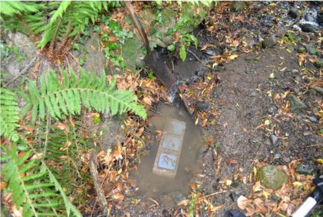
Figure 12 - Concrete block and tiles (in triplicate) positioned in stream at Cavanagrow
