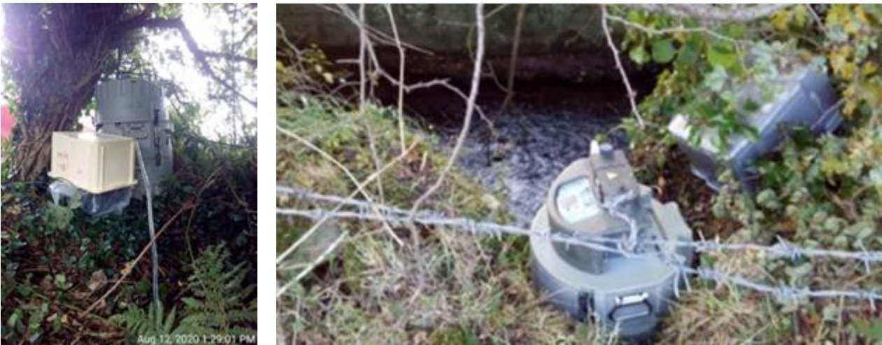
Figure 9 - ISCO 24 hour auto-samplers positioned at the Blairstown Stream, Liscooley.
