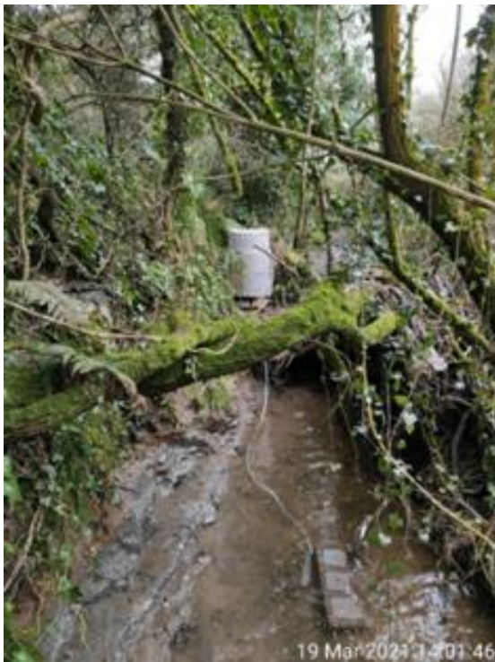
Figure 11 - ISCO auto-sampler positioned upstream at Cavanagrow (block and tiles in foreground).
