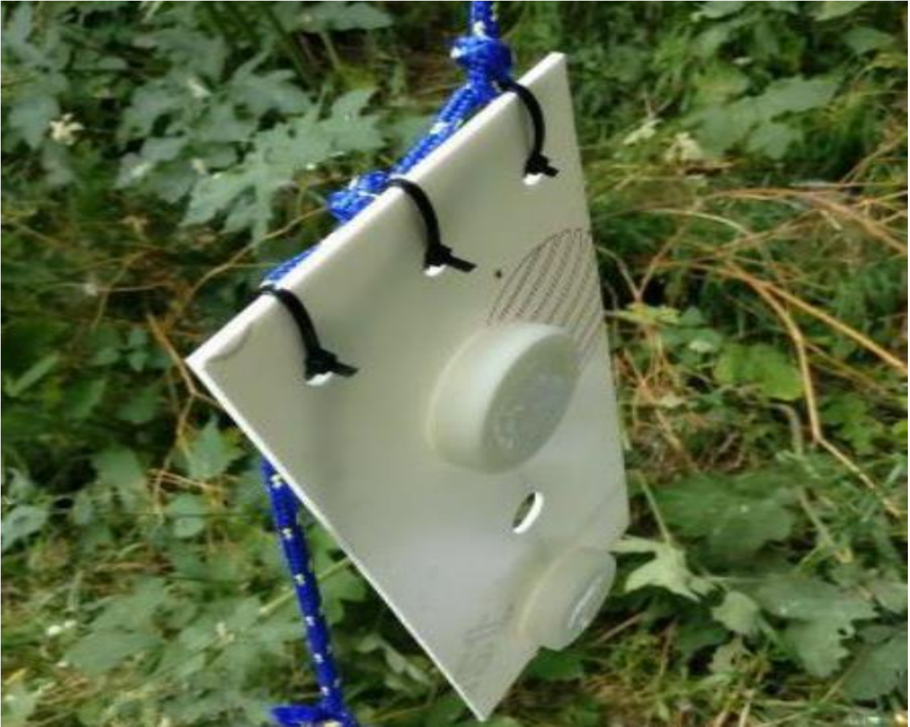
FIGURE 8: PLASTIC CAGING HOUSING CHEMCATCHER AND USED IN METAL ANALYSIS
