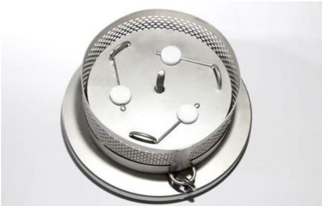
FIGURE 7: PHOTOGRAPH SHOWING INTERNAL PLACEMENT OF CHEMCATCHER RECEIVING DISKS ON A LAYER
