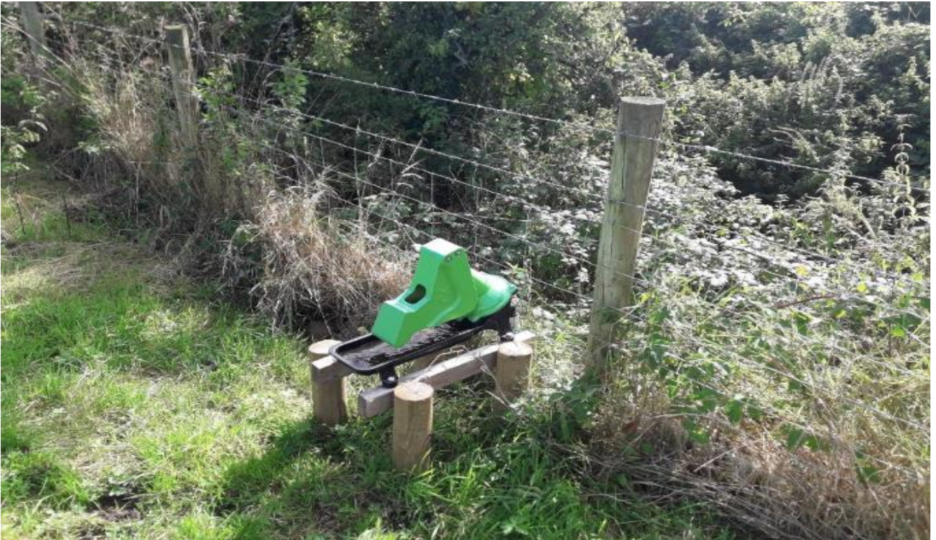
Figure 69: Pasture Pump providing alternative water source for livestock.
