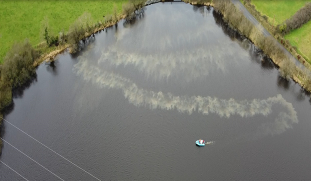
Figure 7 - First sweep of the boat dispensing alum on Corcaghan on 19/01/22.
